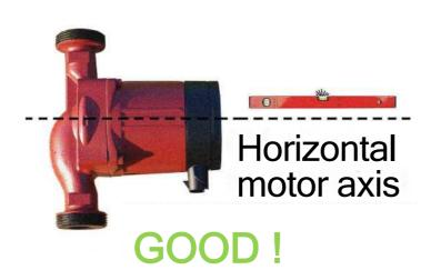
The pump must be installed in such a manner that its shaft is in a horizontal position. Ports can be in a different position than shown in this picture, however, the motor shaft must always be in a horizontal position.
