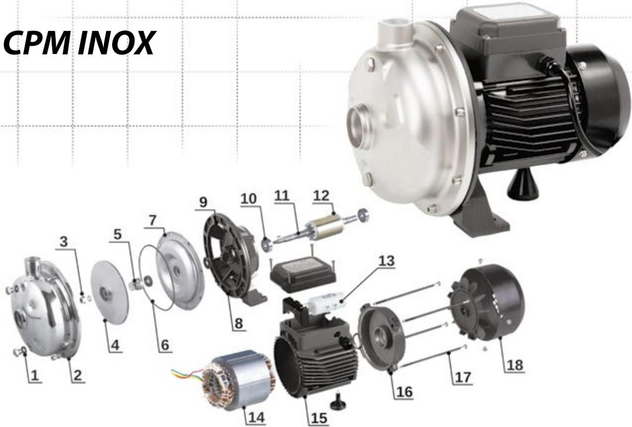
Single-stage non-self-priming centrifugal pumps designed for pumping non-aggressive liquids with non-abrasive and non-absorbent solids content of 0.27 kg/m<sup>3</sup>. The maximum temperature of the pumped liquid is up to 60°C. The pump motor is provided with thermal protection mounted in the motor winding. Hydraulic parts that come in contact with water are made entirely of stainless steel.
