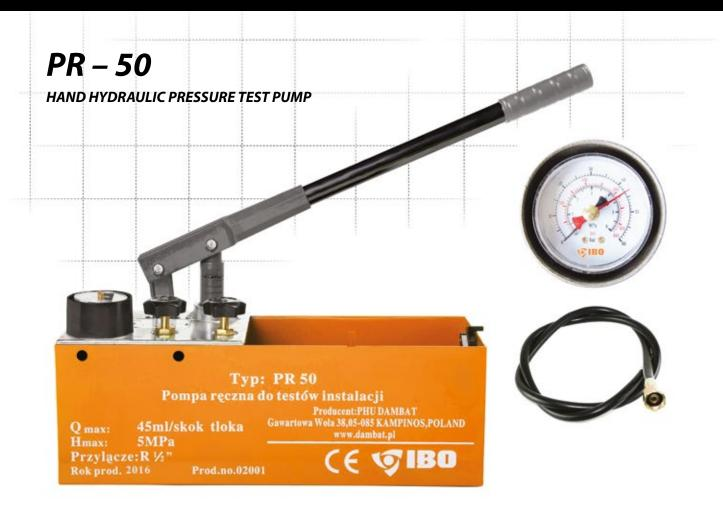
The PR-50 hand pump is a piston pump designed for pressure testing of system tightness and for filling solar system. The main advantage of the pump is that it can be used without access to electric power.
