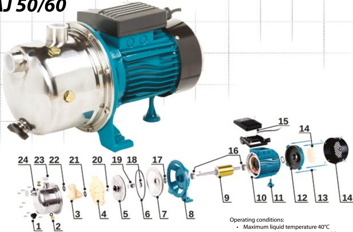
Single-stage self-priming centrifugal surface pump equipped with the Venturi tube system for increased suction capacity, designed for pumping of clean cold water from own intakes and for increasing pressure. Sections of pump body and shaft that come in contact with water are made of stainless steel (INOX design). The pump has a power cable with a plug. The pump motor is provided with thermal protection.
