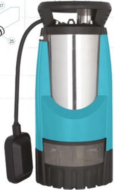
A series of high pressure submersible pumps for irrigation. The pumps have a stainless steel housing and multi-stage hydraulics. The pumps have a cooling jacket so that they do not have to be fully submerged. A filter screen fitted in the bottom of the pump allows water to be pumped down to 10 cm. Both Multi IP INOX pumps are equipped with a float switch for automatic pump control. Like IPE and IPK pumps, all pumps are supplied with thermal protection mounted in the motor winding.
