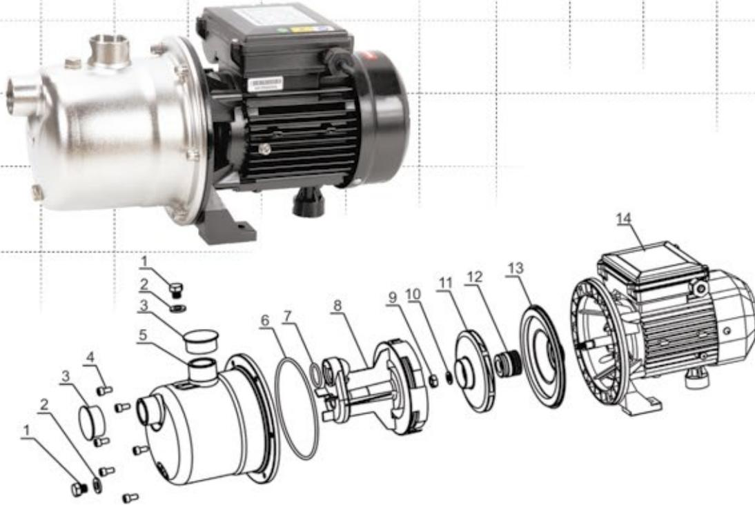
The pump for pumping of clean cold water from own intakes and for increasing pressure. BJ 40/55 is a single-stage self-priming centrifugal surface pump equipped with the Venturi tube system for increased suction capacity. Sections of pump body and shaft that come in contact with water are made of stainless steel (INOX).
