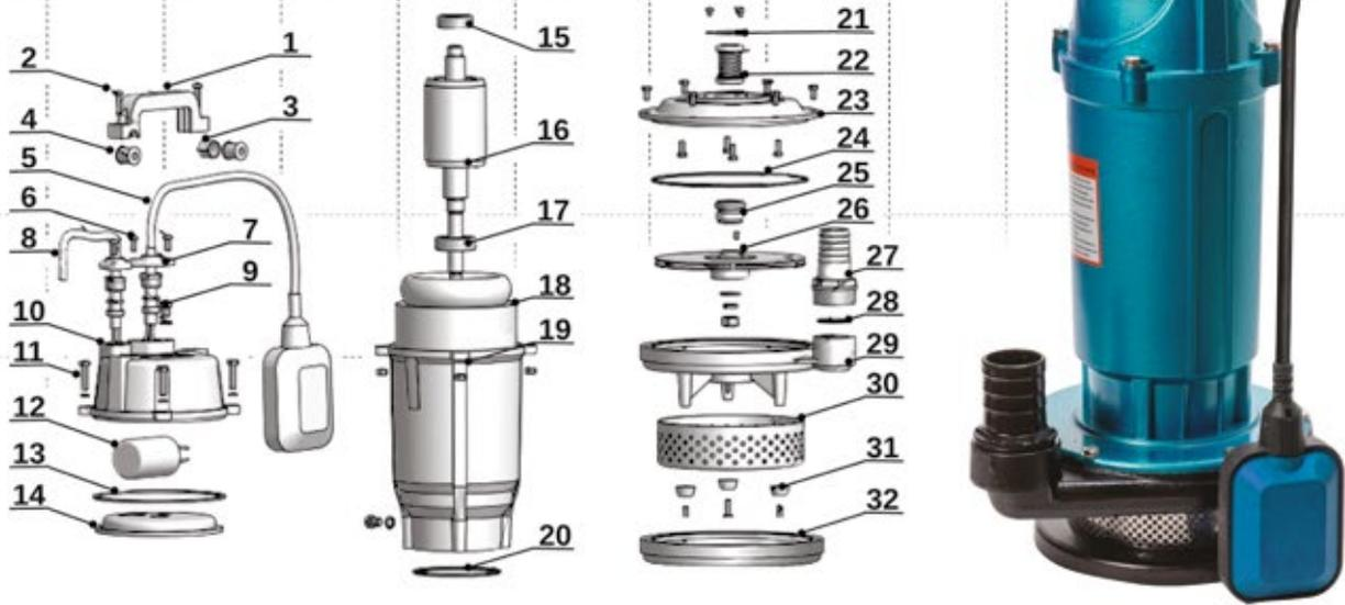
Submersible pumps designed for pumping clean and slightly contaminated water. The motor housing is made of aluminium and the motor is equipped with thermal protection mounted in the winding. High pressure is a special feature of the WQX series pumps. Pump operation is controlled by a float switch. The WQX 250 are available with and without the float switch.
