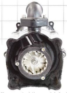
The UP60/80 pumps are equipped with a two-stage hydraulics to increase the maximum pressure. An important feature of KRAKEN 1800 is a multi-channel disk cutting system designed to minimize the risk of clogging. In addition, the outlet is threaded in order to connect a pipeline or fast connection. The pump is supplied with thermal protection mounted in the motor
