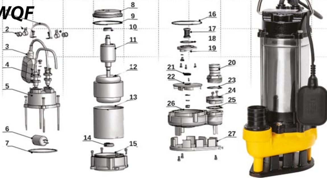
Submersible pumps designed for pumping sewage, dirty water, and water from flooded premises. The pumps are equipped with float switches for automatic pump control. Threaded outlet connection and a set of adapters provide connection of the discharge hose with a hose clamp or fast-connection coupling. WQF pumps are equipped with thermal protection mounted in the motor winding. The motor housing is made of AISI304 stainless steel, and the impeller is made of grey cast iron.
