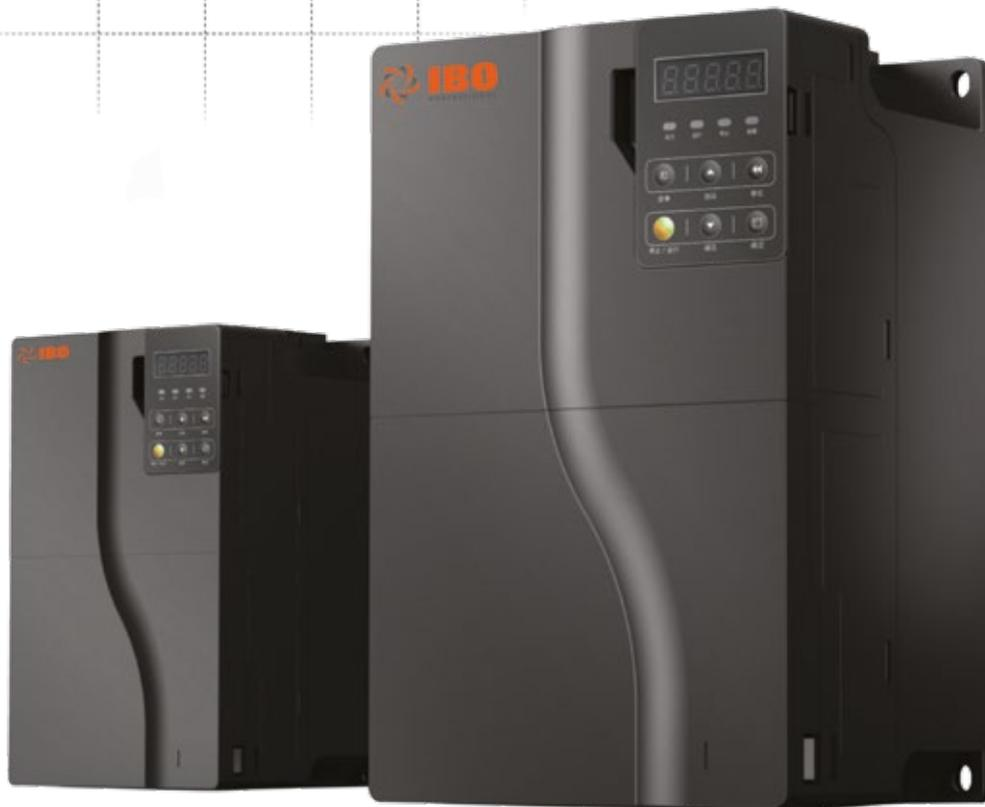
IVR-400T Intelligent Pump Controller is an easy-to-use control and protection device for direct connection of 11 KW to 37 KW (from 15 HP to 50 HP) three-phase submersible pumps, surface pumps, deep well pumps, etc., maintaining a constant, set water pressure by changing the rotational speed of the pump motor.
