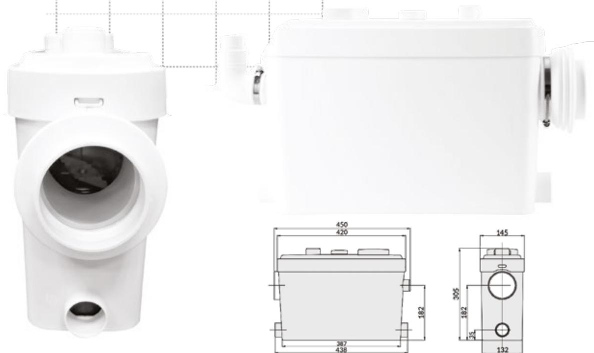
SANIBO B is a toilet pump and cutting system with side inlet. The main application of the pump is to remove sewage from toilets, however, use of three inlets allows to collect sewage from, e.g. bath, washing machine and toilet - one main 100 mm inlet for toilets, two 40mm for shower bases or wash basins, and one 40mm outlet. The pump is exceptionally quiet, so it is an ideal solution for domestic applications. Due to its narrow design, SANIBO B is a perfect solution for concealed frames.
