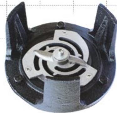
The pumps have an additional chamber in the hydraulic section to increase the maximum pressure generated by the pump. UP-H pumps come with a multi-channel cutting system. In addition, the outlet is threaded in order to connect a pipeline or fast connection. The pumps are available as 3-phase 400V ~ 3 / 50Hz version. The pumps have overload protection on the cable.
