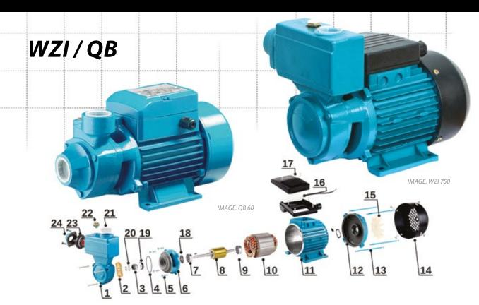
Single-stage self-priming peripheral surface pumps for pumping of clean cold water from own intakes and for increasing pressure. Pump impellers are made of brass. The pump body is made of durable cast iron with the built-in non-return valve. The pump motor is provided with thermal protection.
