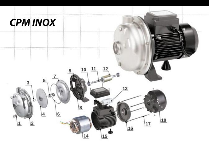
Single-stage non-self-priming centrifugal pumps designed for pumping non-aggressive liquids with non-abrasive and non-absorbent solids content of 0.27 kg/m<sup>3</sup>. The maximum temperature of the pumped liquid is up to 60°C. The pump motor is provided with thermal protection mounted in the motor winding. Hydraulic parts that come in contact with water are made entirely of stainless steel.
