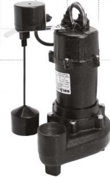
Submersible pumps designed for pumping sewage, dirty water, and water from flooded premises. SN-450 pump is made of cast iron with VORTEX-type impeller. It can pump water with mechanical impurities with particle diameter of up to 20 mm. The pump is equipped with a vertical float switch for easy automatic operation in 25 cm diameter wells. SN-450 pump is equipped with thermal protection mounted in the motor winding.
