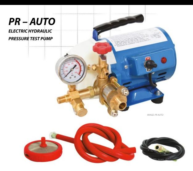
Electric pump designed for pressure testing of system tightness and for filling solar system. The pump's electric motor makes its use exceptionally easy and comfortable. The pump comes with a liquid container, suction hose, high pressure hose, overflow hose and suction filter. Unlike the PR AUTO hand pump, it can also be used to fill the systems with water.
