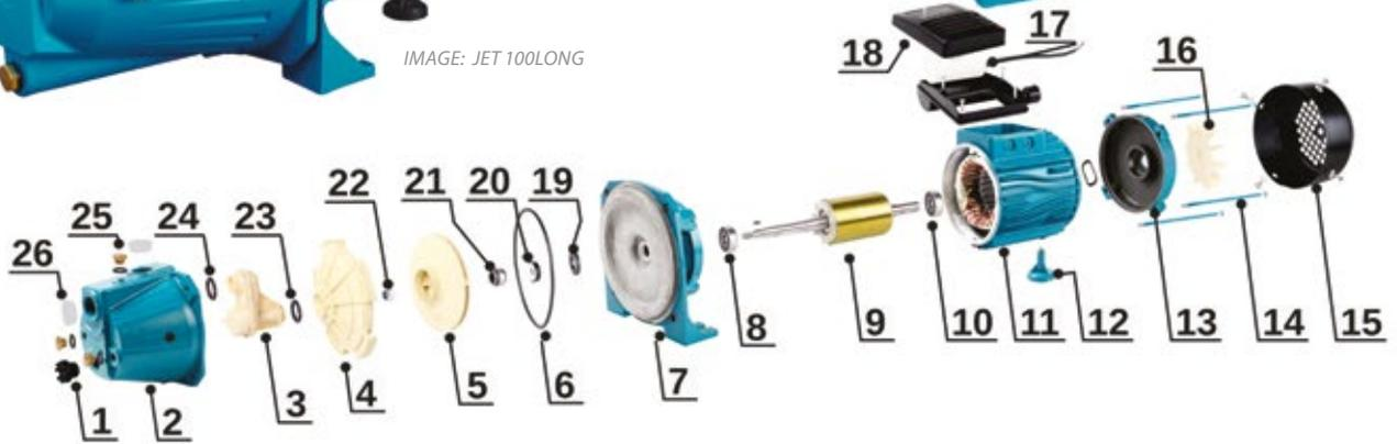
Single-stage self-priming centrifugal surface pump equipped with the Venturi tube system for increased suction capacity, designed for pumping of clean cold water from own intakes and for increasing pressure. The pump body is made of durable cast iron, and the pump motor is provided with thermal protection. The pump has a power cable with a plug. The pump is available with accessories or in the booster set.
