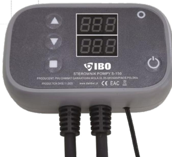
The controller is equipped with 2 LED displays. The current temperature measured by the sensor is displayed as standard on the upper one, while the lower one shows the switch-off temperature. The MENU button toggles the controller into preview mode and switch-on/switch-off temperature settings, as well as the anti-stop function setting.
