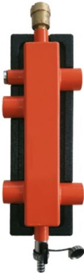
The task of the hydraulic coupling is to separate the boiler circuit from the heating circuit, balance the flows, and keep the pumps running smoothly. Additionally, the coupling protects the boiler against return temperature which is too low.
