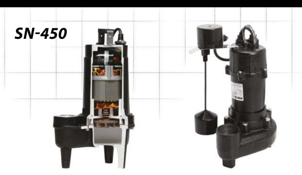
Submersible pumps designed for pumping sewage, dirty water, and water from flooded premises. SN-450 pump is made of cast iron with VORTEX-type impeller. It can pump water with mechanical impurities with particle diameter of up to 20 mm. The pump is equipped with a vertical float switch for easy automatic operation in 25 cm diameter wells. SN-450 pump is equipped with thermal protection mounted in the motor winding.
