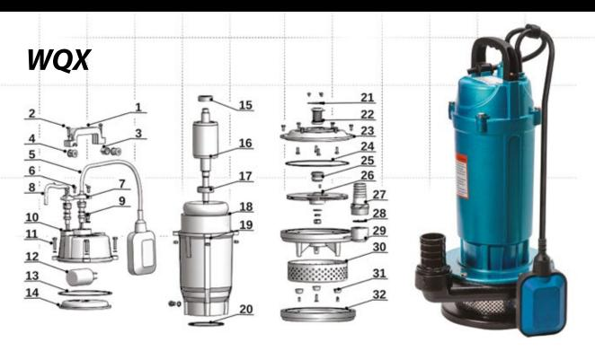
Submersible pumps designed for pumping clean and slightly contaminated water. The motor housing is made of aluminium and the motor is equipped with thermal protection mounted in the winding. High pressure is a special feature of the WQX series pumps. Pump operation is controlled by a float switch. The WQX 250 are available with and without the float switch.
