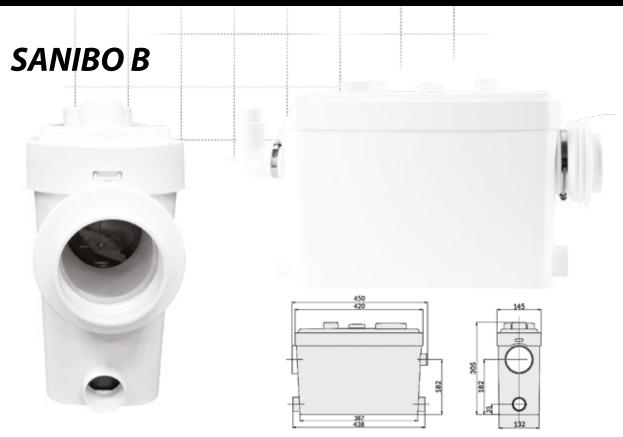
SANIBO B is a toilet pump and cutting system with side inlet. The main application of the pump is to remove sewage from toilets, however, use of three inlets allows to collect sewage from, e.g. bath, washing machine and toilet - one main 100 mm inlet for toilets, two 40mm for shower bases or wash basins, and one 40mm outlet. The pump is exceptionally quiet, so it is an ideal solution for domestic applications. Due to its narrow design, SANIBO B is a perfect solution for concealed frames.
