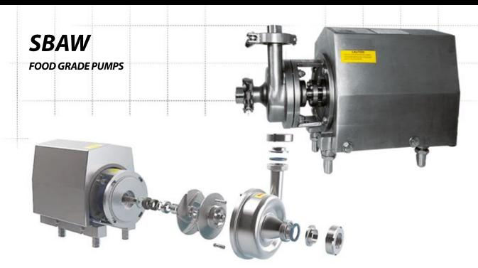
Pumps designed for transporting concentrated or non-concentrated food liquids with up to 50% dry matter content or other food products with a temperature up to 75°C. Centrifugal pumps with open impeller, enclosed motor, and distanced hydraulic body. Inlet/outlet are complete with connections for easy installation. The device has four adjustable legs. SIC/WC (EPDM) mechanical seal. VMQ body seal/
