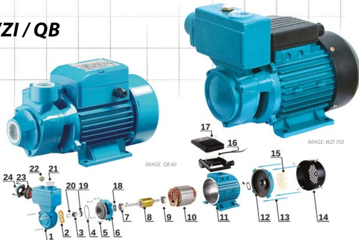
Single-stage self-priming peripheral surface pumps for pumping of clean cold water from own intakes and for increasing pressure. Pump impellers are made of brass. The pump body is made of durable cast iron with the built-in non-return valve. The pump motor is provided with thermal protection.
