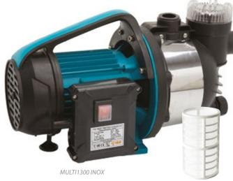
Self-priming centrifugal pump with the built-in screen filter, equipped with the Venturi tube system for increased suction capacity.
