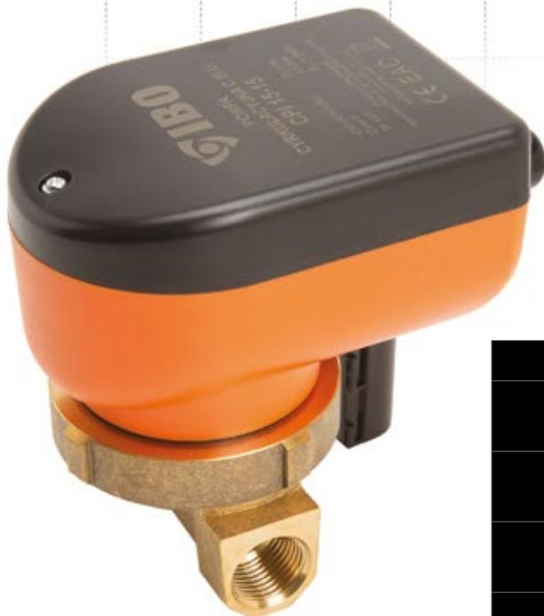
Seal-less circulation pumps designed for forcing hot water circulation. In systems without hot water pumps, after opening the tap, before the hot water starts flowing, cool water remaining in the pipeline will flow first. If a hot water pump is installed, hot water will flow almost immediately after opening the tap. The pump is usually installed upstream the boiler or hot water tank. With years of experience, we have been able to improve previous designs and create the top quality pump.
