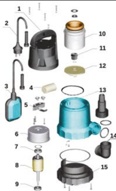
IP submersible plastic pumps designed for pumping clean and slightly contaminated water. The pumps have an outlet connection to which discharge hoses of different diameters can be connected depending on the user's requirements. Small size and light weight make the pumps exceptionally easy to operate and maintain. The pumps are equipped with float switches for automatic pump control. All pumps are supplied with thermal protection mounted in the motor winding.
